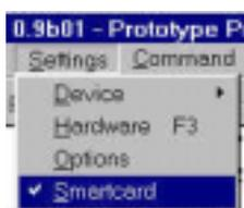
There is one special setting in the programming software. "Smartcard", This setting is intended for Trough PIC programming using a Phoenix or SmartMouse card interface (Mode #0 and #1). This option is to be switched of in MASTERA-II Mode #2 and #3.
