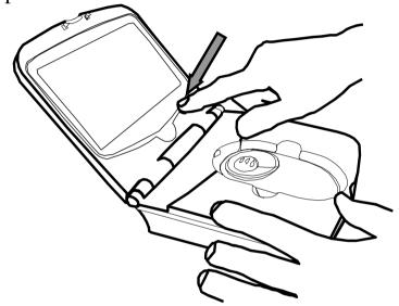
When you place the unit on some text you should see the magnified image on the screen. The base of the main unit is fitted with rollers to allow the entire unit to glide easily over what you want to read. **Note:** the camera "sees" beneath the scroll zoom wheel, bear this in mind when locating what you want to read.
