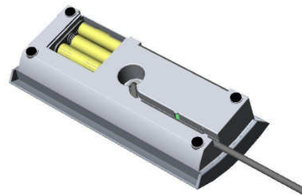
5. Reinstalling the battery housing.
