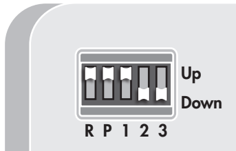
Figure 11 Locating the VIM configuration switches, rubber boot removed
