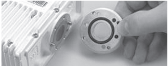
Figure 5 Transceiver & adaptor, showing correctly located adaptor ring
