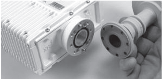
Figure 7 The feedhorn/adaptor interface with adaptor ring
