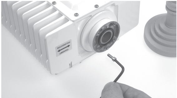
Figure 6 Connecting the adaptor to the transceiver
