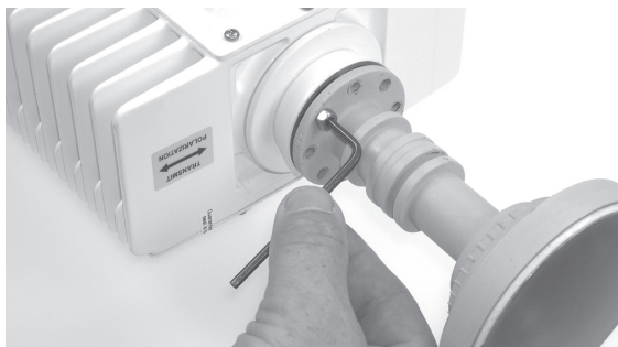
Figure 8 Connecting the feedhorn to the adaptor
