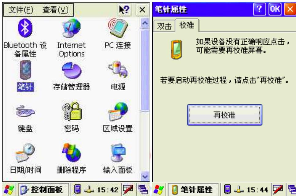
According to the system prompt, use the five-point calibration method to start using touch pen calibration, calibration has finished, it will jump out the window as follows, At this time the location of any point to return to a "Stylus Properties" window, point of "OK" to save.
