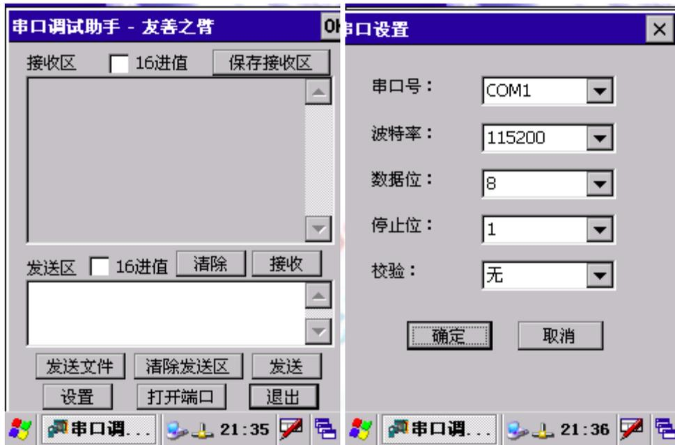
Point of the "Settings" button, open the settings window, set the serial number is COM2, baud rate to 115200, and other established home figure (upper right), determined to return to the main window.
