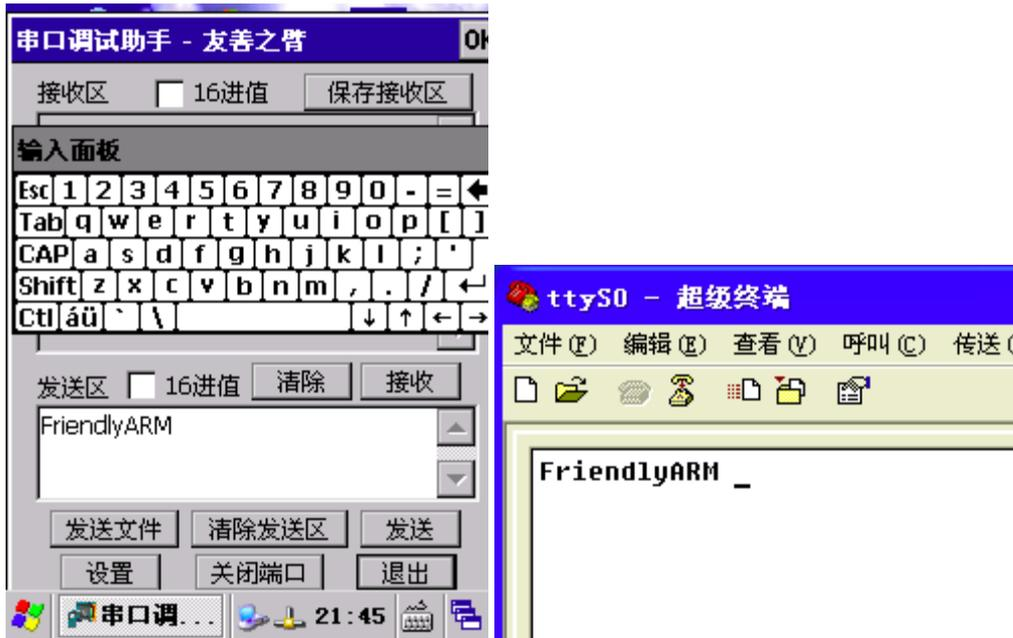
Then, in the serial port of the main window debug aides point "receive" button (the button will change to "not to receive"), in PC-side input terminal of the serial number of characters (via HyperTerminal cannot be seen), the import of the same time, we see the importation of character development board in the reception serial debugging assistant district showed that figure:
