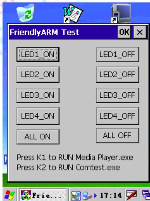
Click the process button, can control the development of the four on-board LED's light and out.
