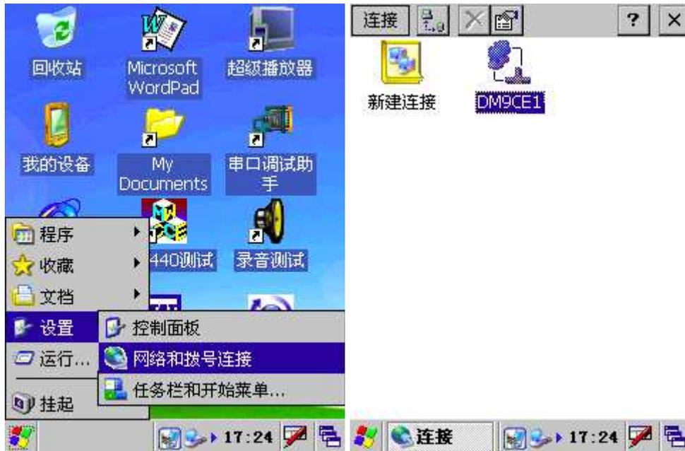
Double-click DM9CE1, open the settings interface, under the plan is the default configuration, you can install the actual network environment settings.
