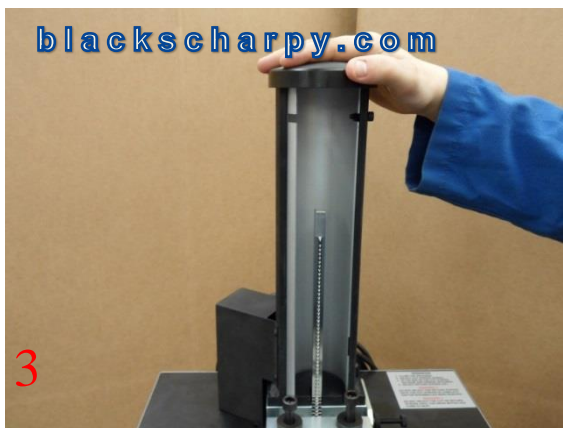
3 Open broach guard shield and determine feeler gauge thickness for broach type being used, from Table 2
