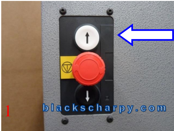
1 CNB31– Press “up” to raise broach to upper position, with no specimen loaded
