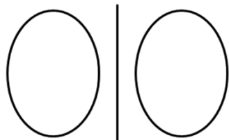
Fig 2. Variable transformer isolation symbols
