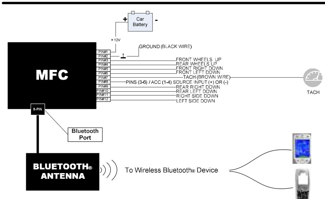
Figure 9: MFC Example: Setup as Hydraulics Controller
