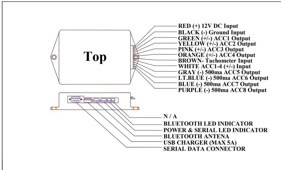
Figure 5: MFC CONNECTOR DIAGRAM
