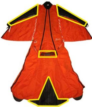
**New low drag materials** - beside regular ZP Balloon used in previous wing suit designs, Vampire V-1 is for the first time utilizing Dacron on the wing leading edges and on the leg wing trailing edge. Dacron, the most popular material for hang glider skin, is light, durable, and easy to shape, has low drag characteristics and better maintains the desired airfoil shape.
