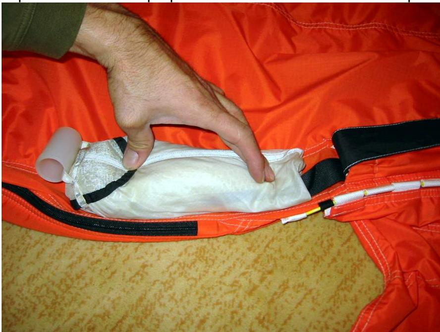
Figure 2 Rolled pilot chute
