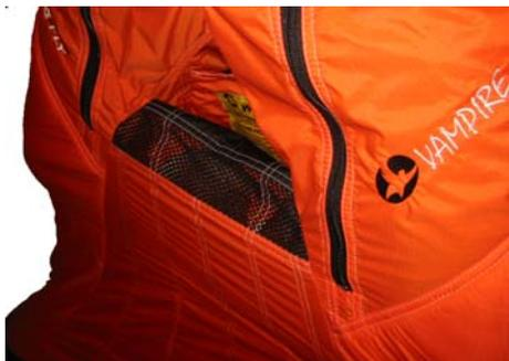
**Leg wing leading edge** is also reinforced with Dacron for extra stiffness and smoother shape, supported by one layer of the foam covered by F-111 on the inside. The air inlet has also been redesigned, maximising pressurization without sacrificing performance.
