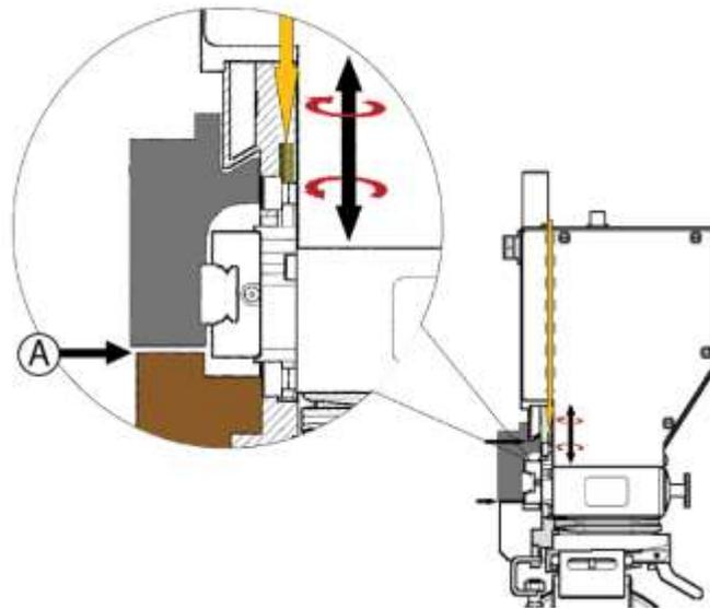
3. Insert a .002" feeler gauge at A (between the guide bar and the brown stop block).
