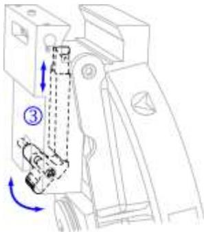
4. Manually actuate the sidestroke key and the cam (3) parts, checking for free and smooth movement. If parts are sticking, call Tidland Customer Service for assistance.
