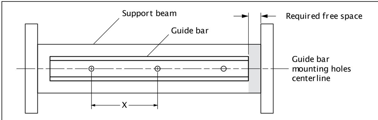
Determine the center-to-center distance between the mounting bolt holes (**X**) on the guide bar.
