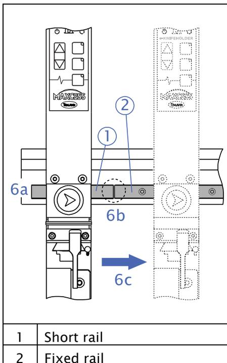
1. At the mounting end only, locate and remove the #10-32 screw on the face of the guide bar.
