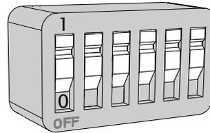
2. Find the corresponding number for your knifeholder in the table below. With a small flat blade screwdriver, carefully move each switch to the correct OFF or ON position.
