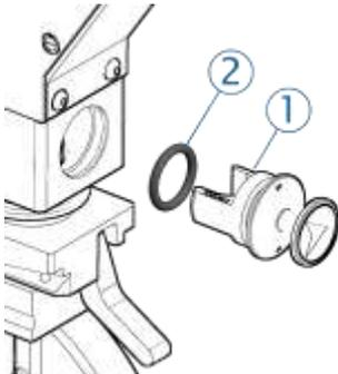
If the cant key (1) becomes loose in the body or if cracks in the o-ring (2) are visible, replace the o-ring. Lubricate the new o-ring and the cant key o-ring groove. Use only *Parker Super O-Lube* (no substitutes).
