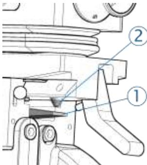
During operation, the side-stroke lever (1) is activated by the side-stroke actuator (2) located at the cartridge-to-dovetail interface. If this area becomes clogged with dust and debris, the actuator can become stuck, resulting in loss of side-stroke.
