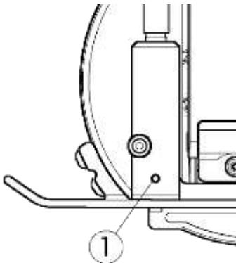
To adjust the guard for a closer fit to the knife blade, turn the M5 adjustment set screw (1) clockwise until the guard touches the blade, and then back off one-quarter turn.
