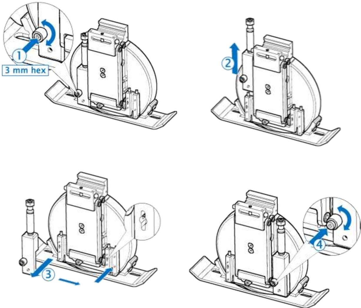
Before reinstalling the blade cartridge on the knifeholder, remove dust and debris from the dovetail interface components.
