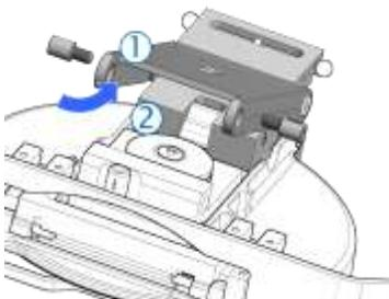
2. Using 4 mm hex drive, remove two pivot pins and lift up the cartridge strut (1).
