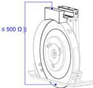
6. Use an ohmmeter to measure for  $\leq 500 \Omega$  between the top of the cartridge dovetail and a point on the knife blade. Rotate the blade and measure in several places.
