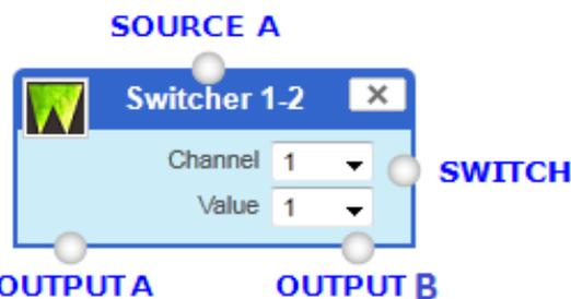
Switcher 1-2: Controllable Switch operator, when the trigger channel (Switch) is greater than the set value, OUTPUT B is output, in other cases OUTPUT A is output.
