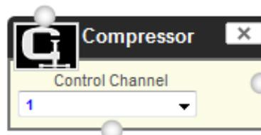
Compressor proportionally reduces all channels of the input according to the value on the control channel.
