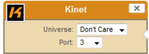
**Kinet Stream:** For example: You can connect Kinet Stream to an Art-Net Stream to convert and output as Art-Net. (Kinet stream is supported as input only)
