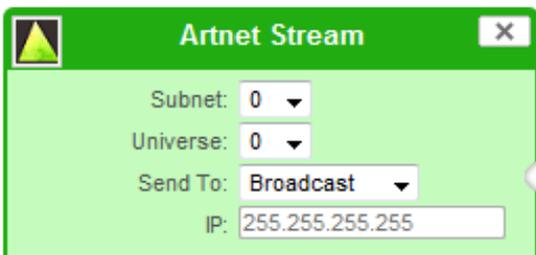
**Art-Net Stream:** "Send IP address": is the destination address used when the stream is sending data only.
