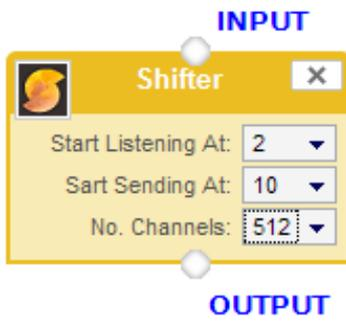
Shifter: can be used to shift a number of channels to another spot in the INPUT DMX frame
