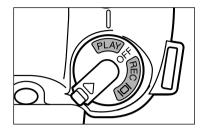
Turn the camera's Main Switch/Mode Selector dial to PLAY, then press the MENU button on the back of the camera.
