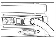
When the camera is the only connected SCSI device: Attach the other end of the SCSI cable to the computer's SCSI host adapter.
