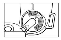
Turn the camera's Main Switch/Mode Selector dial to PLAY, then press the MENU button on the back of the camera.
