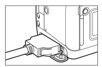
Align the 50-pin Wide SCSI cable connector to the camera's SCSI connector, and press it in firmly until it clicks into place.
