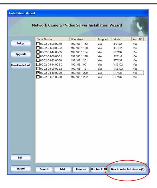
For more detailed usage of the Installation Wizard, please refer to the user's manual of the Installation Wizard included in the product CDROM to find the location of the Network Camera. There may be many Network Cameras in the local network. Users can differentiate the Network Cameras with the serial number. The serial number is printed on the labels on the carton and the back of the Network Camera body. Please refer to the user's manual of Installation Wizard for detail.
