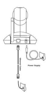
Please verify that your product package contains all the accessories listed in the foregoing Package Contents. Depending on the user's application, an Ethernet cable may be needed. The Ethernet cable should meet the specs of UTP Category 5 and not exceed 100 meters in length.
