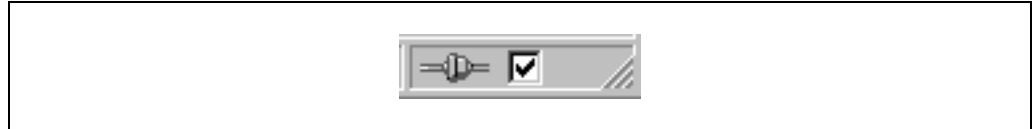
Fig. 11: Status bar with symbols for “connected” and “configuration verified”
