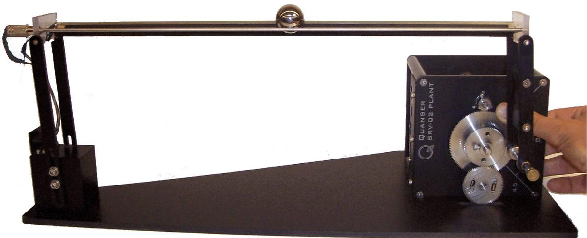
Figure 7: Calibrated BB01: ball is balanced when centered on beam.
