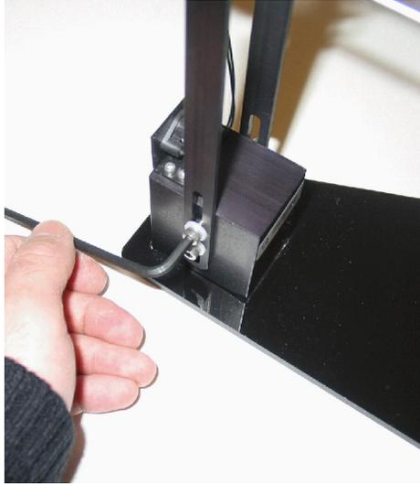
*Figure 8: BB01 calibration: tighten support arm screws once beam is balanced.*
