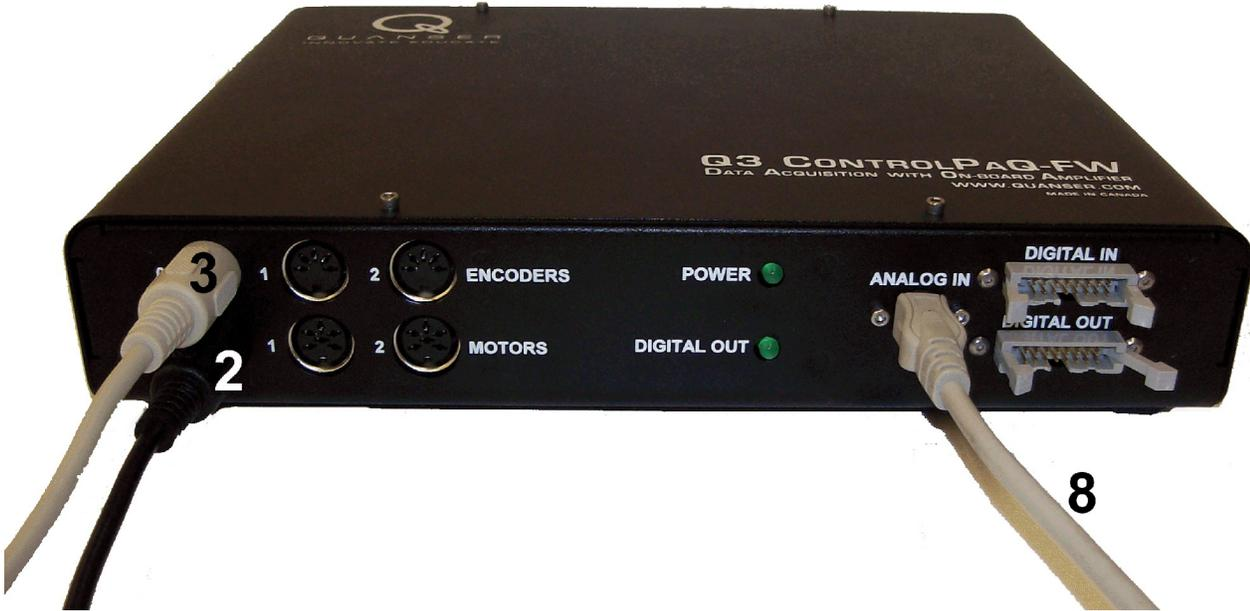
Figure 19: Connections on the Q3 board from the Analog 2:1 Buffer box and the BB01.
