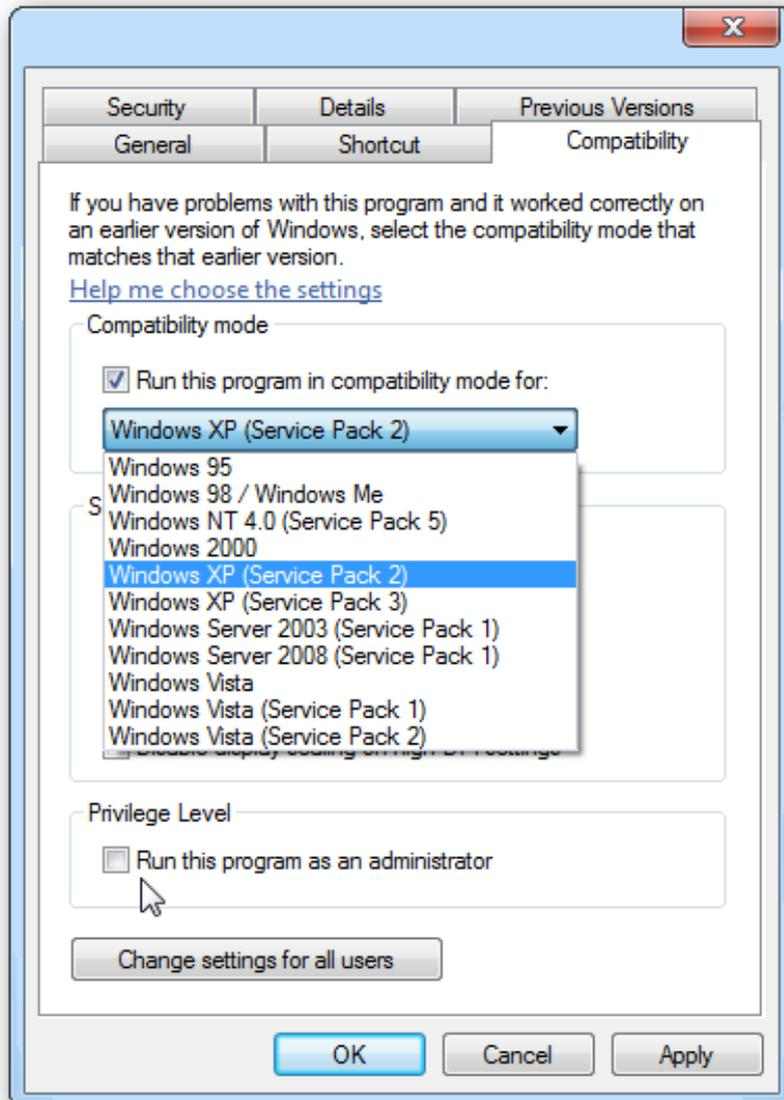
Figure 10 - ISUScore2FS - Run program in compatibility mode
