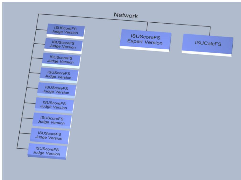
Figure 1 - System Layout of a level 2 system (no video replay)
