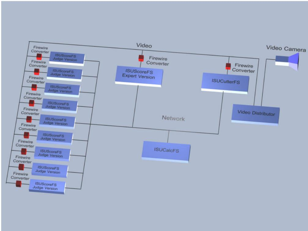
Figure 3 - System Layout incl. video replay for the Technical Panel and all Judges
