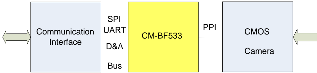
Figure 5-2: Block Diagram – Mini Camera Module
