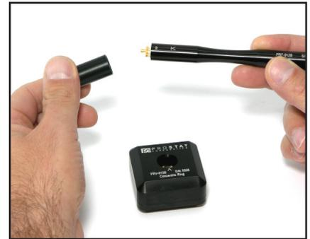
Figure 5: Remove Probe Cover
