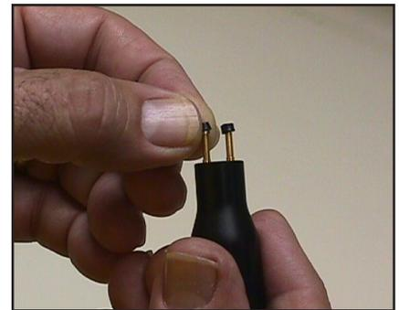
**Figure 9: Installing Conductive Rubber Electrode “Boots”**
