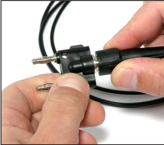
**Figure 3: Connect Cable to Banana Converter**
