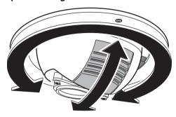
The Alien 05 is supplied with a diffuser filter installed. This ensures a soft illumination when illuminating close objects. When illuminating objects at greater distances, it is recommended that you remove the diffuser filter. See "Removing the diffuser filter" on page 14.
