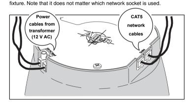
4 Once the cables are connected, insert the Alien 05 into the mounting hole.
