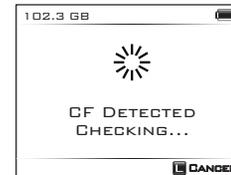
The data on the memory card is compared with the data stored on the NVS1501 hard disk to determine whether it is new data or if the data or a portion of the data has already been stored on the NVS1501. According to the comparison result, the NVS1501 operates as follows:
