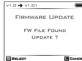
If valid firmware is found at the specified location, the NVS1501 indicates a “FW File Found” message on the LCD. Confirm the firmware upgrade by pressing the control key briefly [S].
