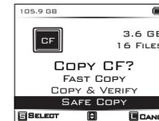
The NVS1501 will make a new folder on the hard disk and copy all the files and folders in the memory card onto the internal hard disk. The contents of the memory card will not be deleted.
