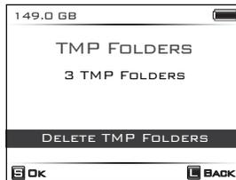
If the TMP folder exists inside the [NVSPRO] folder, then the number of TMP folders will appear on the LCD. Press the control key briefly [S] to delete the TMP folders.
