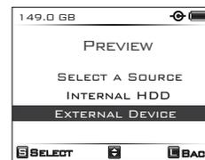
The NVS1501 supports the preview of video files stored on an USB external hard drive—as well as video files stored on memory cards such as: SDHC, SDXC, MS, MD and CF.
