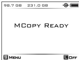
The remaining operation is the same as the “XCopy ready” mode. This mode can be exited by holding and pressing the key or by removing the USB cable from the NVS1501.
