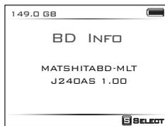
If a Blu-ray drive is properly connected, the NVS1501 will detect it and display the information as shown in the figure. Press the control key briefly [S] to go to the next step.
