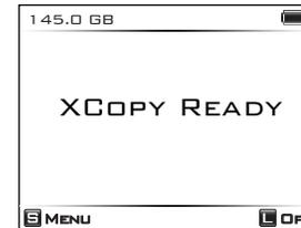
After checking the system, the NVS1501 goes into [XCOPY ready] mode. You can copy a memory card in this mode.
