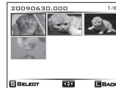
The NVS1501 shows a list of video files contained in the selected folder as thumbnails. Unsupported video files are shown with an [X] mark. Select a video clip for preview using the up/down/left/right function of the control key.
