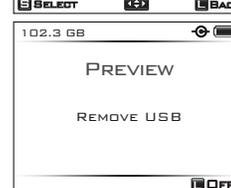
If you select “Back” by pressing and holding the control key, then a “remove (device type)” message will appear on the LCD display. Once the cable or memory card has been removed, you will automatically be returned to the main menu.
