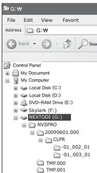
Back up data is stored in the "NVSPRO" folder. This folder is created automatically. The NVS1501 generates a new folder for each memory card copy. The name of the folder is determined by the shooting date.
