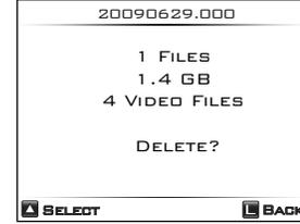
The NVS1501 will ask you twice to confirm the delete operation. (If you do not want to delete, press the button for more than 2 seconds to go back to the main menu.) Push the control key up and down to confirm the deletion.
