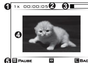
The NVS1501 will show a preview of the video file at reduced resolution. The user can select play/pause by pressing the control key. The user can also adjust the preview speed by pushing the control key to the left/right.
