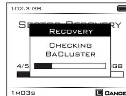
The data will be copied to a safe area on the internal hard drive—while the faulty sectors are being filled with dummy files.
