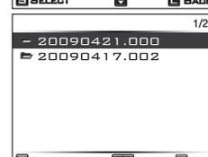
(2) If an USB hard drive is connected, the NVS1501 will detect and analyze the backup folders. The NVS1501 will then display the backup folders as in the figure. The rest of operations are the same as previewing from the internal hard drive
