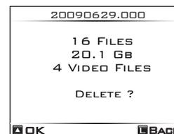
The NVS1501 will ask you twice to confirm the memory card deletion operation. If you do not wish to proceed with deleting the data from the memory card, press the control key for more than 2 seconds to go back to the main menu.
