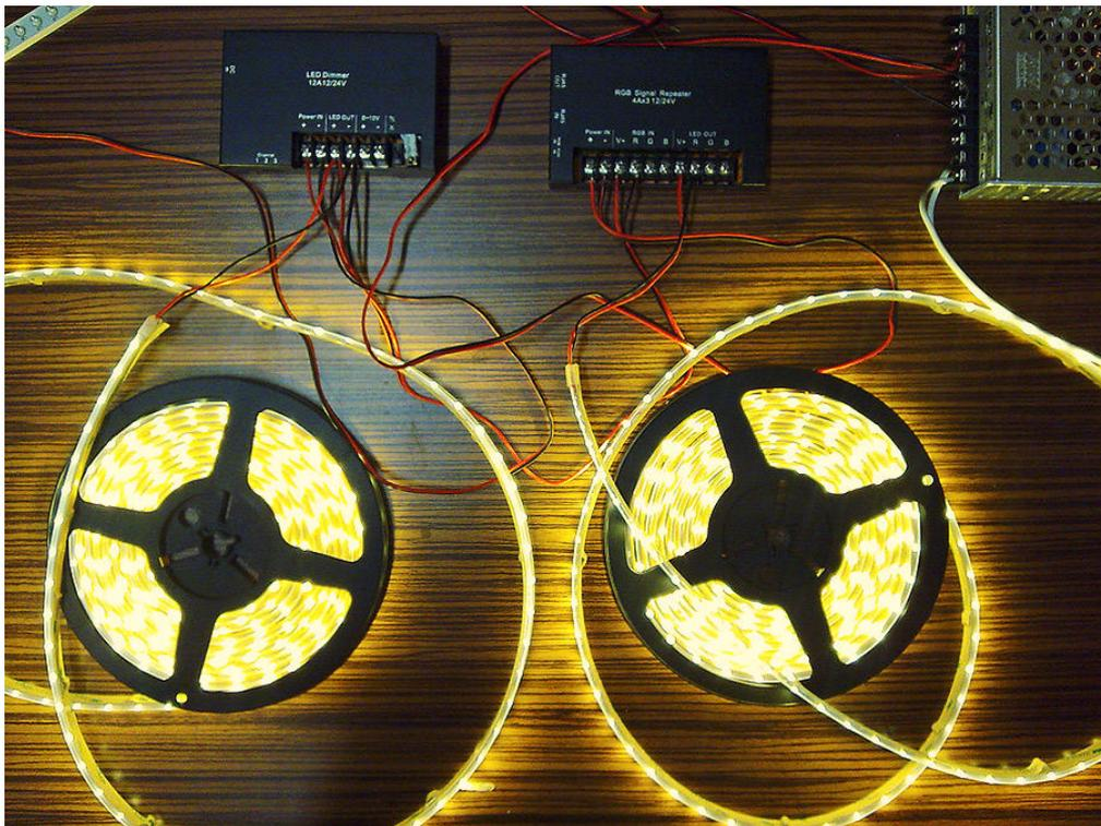
Note : When connecting to repeater, the negative of LED IN and LED OUT have to connect to the same channel.
