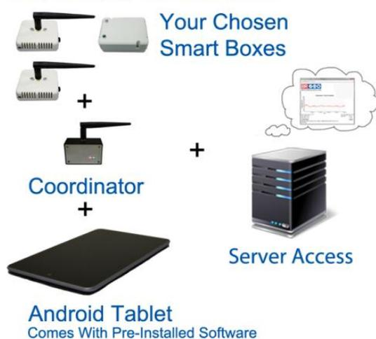
The Custom Kit comes with a pre-installed and configured logger and is ready to work out of the box. All that is required is to power up the devices to get instant results and for server access and historical data configure your Wi-Fi connection with internet connection.
