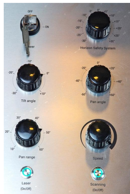
figure 7: SeaBird Saver display panel. With the Horizon Safety system, Tilt angle, Pan angle, Pan range, movement Speed, laser on/off and scanning on/off dials and buttons
