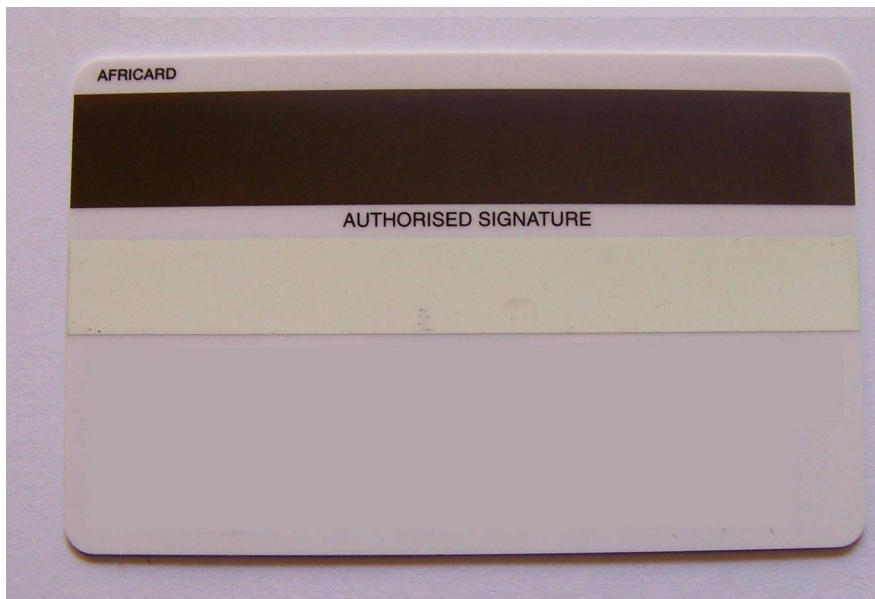
Figure 3.1: A plastic magnetic stripe card
