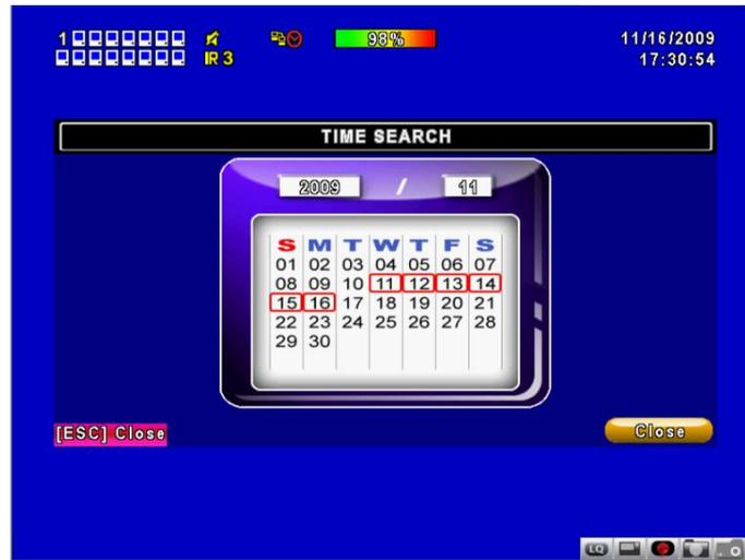
Click “date” to display recording time of that specific date with time bar. You can change time (hour/minute/second) or click on a specific time of time bar by mouse then press “ok”. DVR will playback the selected recording data.
