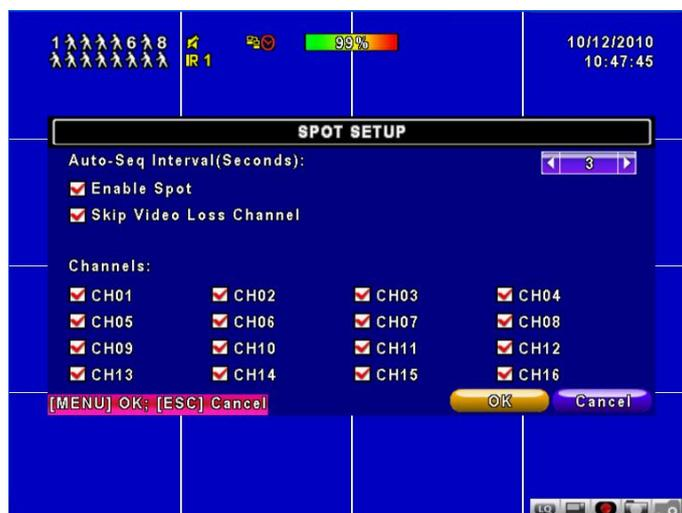
**DVR's Main Monitor output signal, do the main screen output or switch SPOT mode output**
