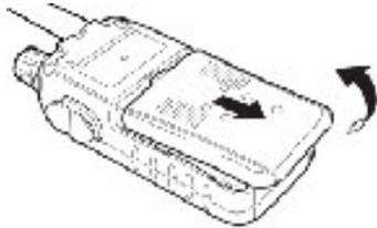
Slip the battery cover backward at the back of the interphone, and then get it from the body of the interphone.
