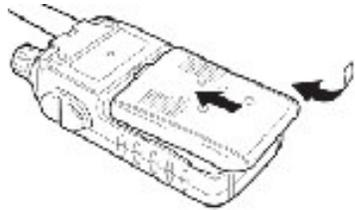
The lock tongue of the battery cover aims at the lock groove, and then Make it tight at the right position.
