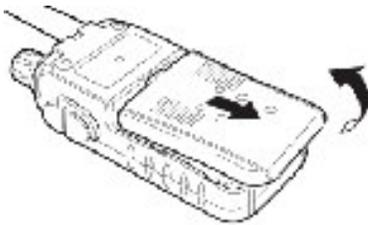
The lock tongue of the battery cover aims at the lock canal of the interphone, and then makes it tight at right position
