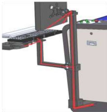
Fig.3-8 The line sketch map of display, keyboard and mouse (red is the connection)
