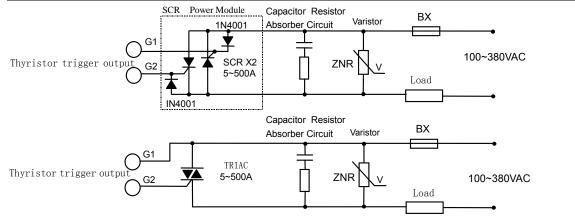
Note 1: According to the voltage and current of load, choose a suitable varistor to protect the thyristor. A resistor-capacitor circuit (RC circuit) is needed for inductance load or phase-shift trigger output.
