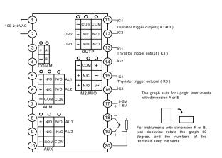
Note 4: When main output selected linear current or SSR voltage, output form terminal 13+, 11-,
