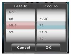
Figure 23 - Heating and Cooling Setpoint Editors
