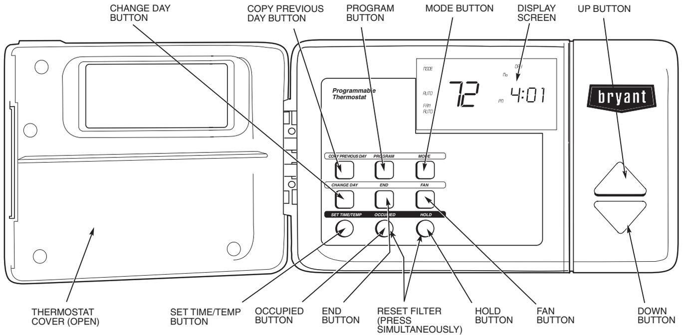
Fig. 2 — Thermostat Display and Programming Buttons
