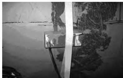
FIGURE 19: Transducer QMP-F05 (500 kHz) for large pipes – Mounting with textile tape.
