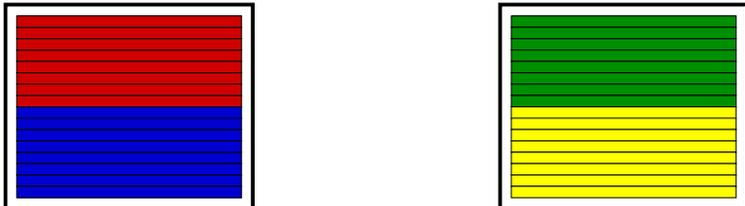
Figure 3-2. Field Order, Bottom Field First Transmitted
