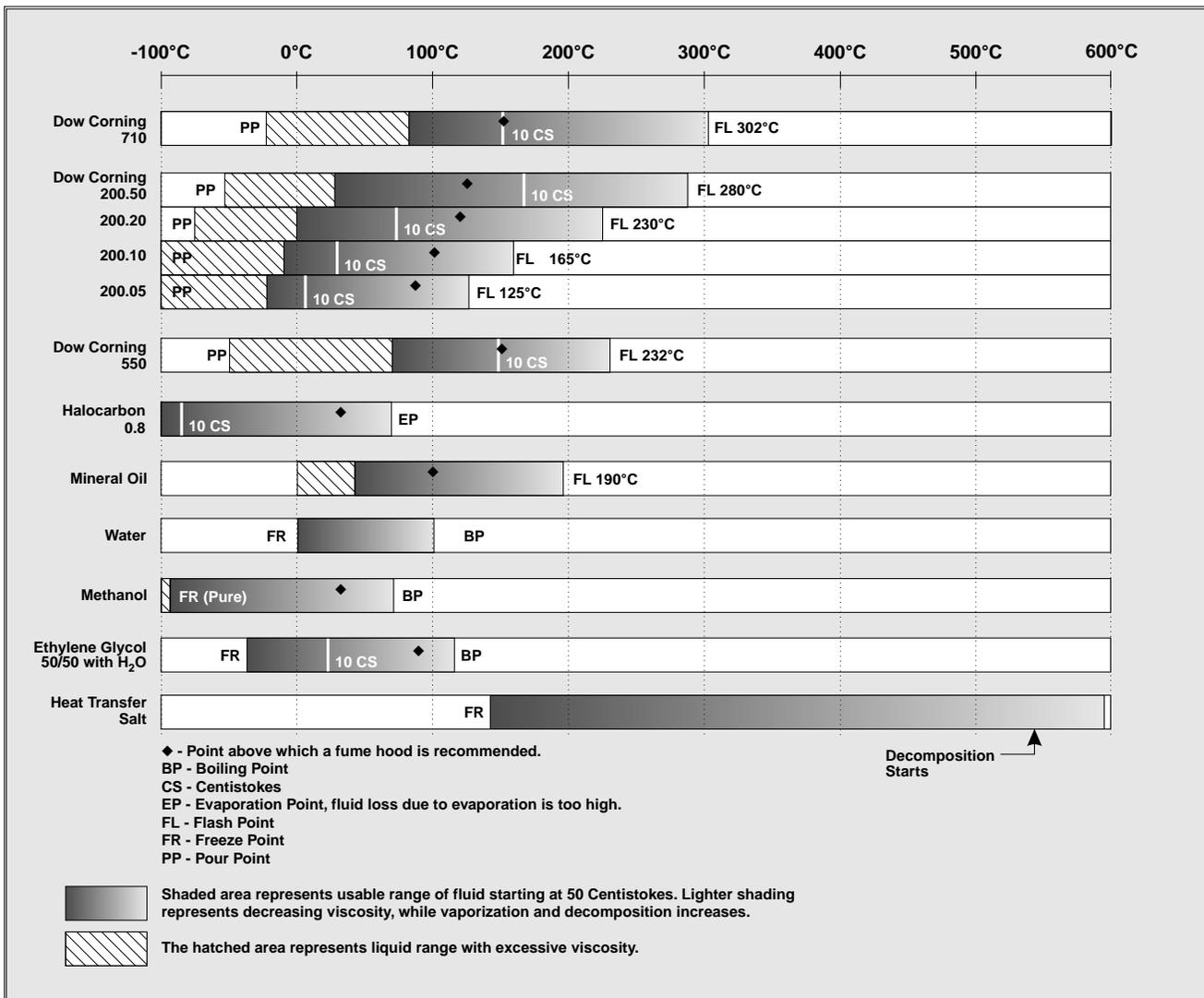
Figure 3 Chart showing usable range of various fluids
