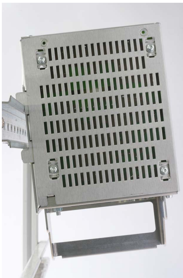
Figure 5-1 Mounting on the DIN rail based on the example of a SCALANCE X204RNA EEC
