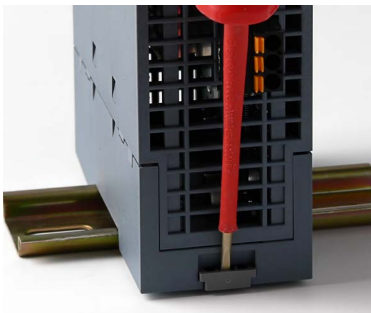
Figure 5-3 SCALANCE X204RNA removing from a DIN rail (35 mm)
