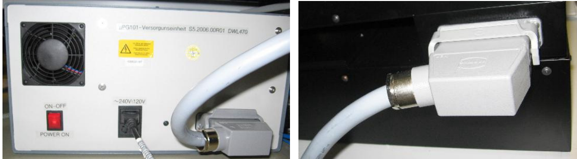
Figure 6: System power connection from supply unit (left) to lithography system (right)
