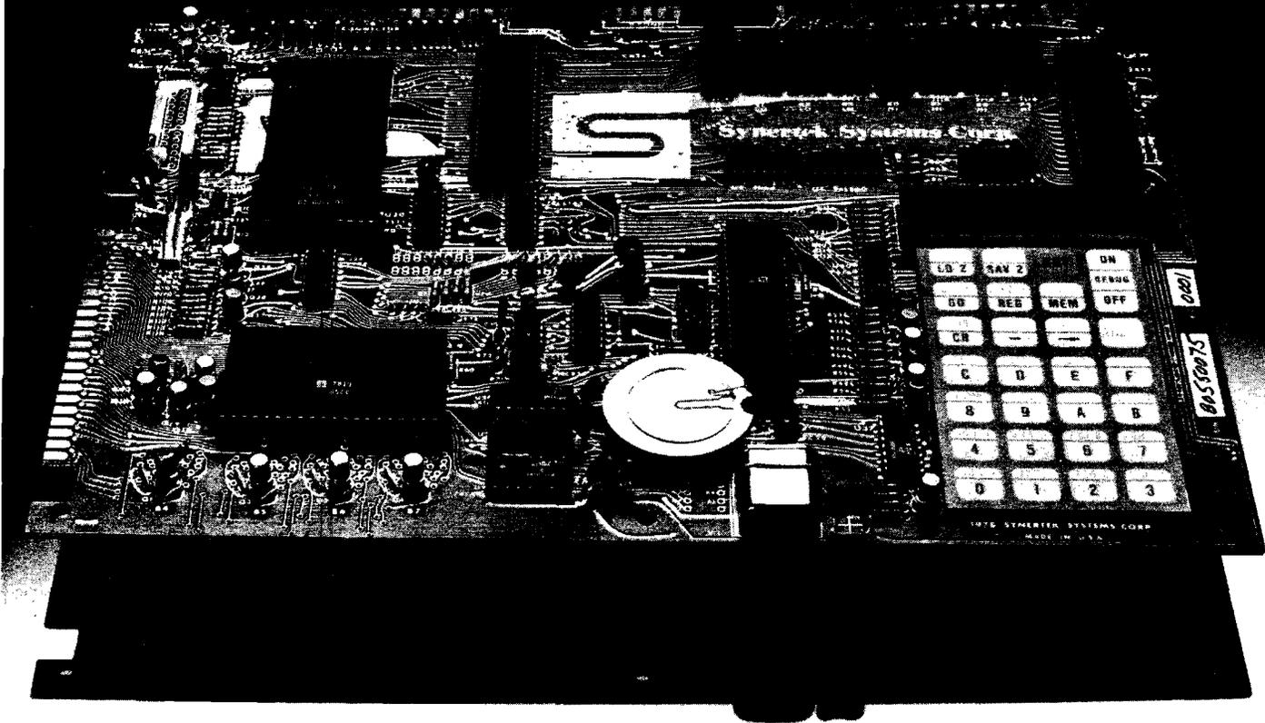
In performance. In quality. In availability. OEMs, educators, engineers, hobbyists, students, industrial users: Our Versatile Interface Module, SYM-1, is a fully-assembled, tested and warranted microcomputer board that's a true single-board computer, complete with keyboard and display. All you do is provide a +5V power supply and SYM-1 gives you the rest—and that includes fast delivery and superior quality.
