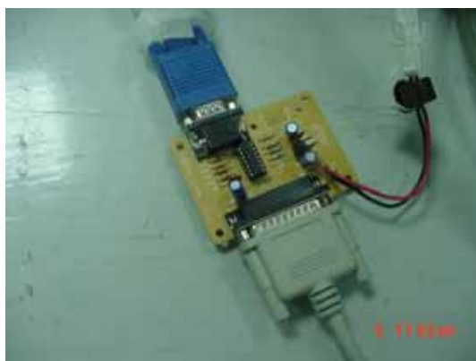
Connection of DDC-writing instrument for VGA.
