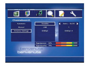
The Signum is programmed for Astra Satellite but you can set up the antenna installtion as well as the channel search for other satellites.
