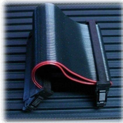
Figure 4 –80 Pin Connector
