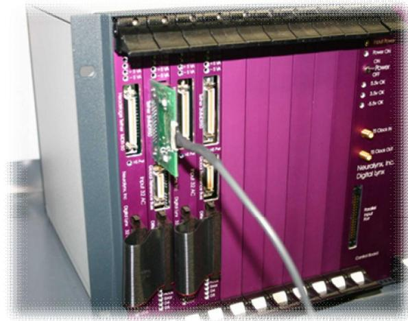
**Figure 6 Tether Adapter Connection**
