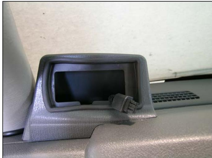
6. Insert the *Evolution* securely into the rubber grommet of the pod. Final installation is shown. Secure any excess cable under the dash to prevent interference with pedals.
