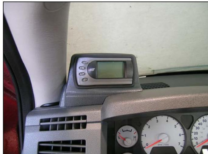
7. With the Pod and *Evolution* securely in place, turn the ignition key ON. Then plug the cable into the OBDII connector. The Evolution logo will be displayed followed by a disclaimer. The *Evolution* logo will display followed by a warning and compliance directive. To indicate you accept and acknowledge the warning and compliance, press the [ENTER] button
