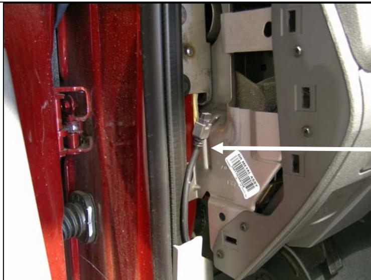
Run the cable inside of the access panel.
