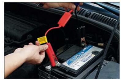
■Plug the cord of the jump cable into the jump starter socket and then press the power button. Make sure that 2 SF-1 indicator lights are bright
