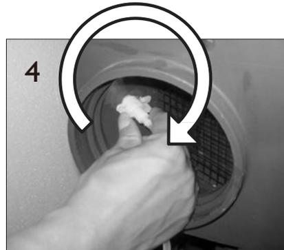
4 Turn the connector 90 degrees clockwise until it is locked in place.
