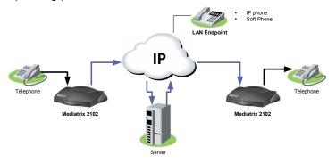
Calls Involving an Access Device and a LAN Endpoint The following examples illustrate how a phone/fax connected to a Mediatrix 2102 access device can communicate with a LAN Endpoint on the IP network.
