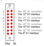
2) With DB37-CC4-16 converter, ports of  $E1/1 \sim E1/8$  are as the following diagram:
