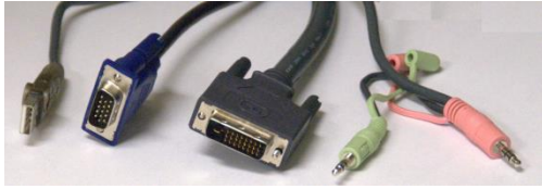
Figure 3. Cable connectors to the personal computer. You will need to connect one of the video ports (DVI or VGA) and the USB cable. If you want to play any sound, you will also need to connect the green connector (🔊) to your audio output port. If you want to record speech to your computer, you will need to connect the pink connector (🎤) to your microphone port. Note that the audio and
