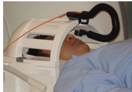
Figure 10. The speech recording microphone, the flex-boom and stand to mount. The microphone should be as close to the subject's mouth as possible, but without touching the subject.
