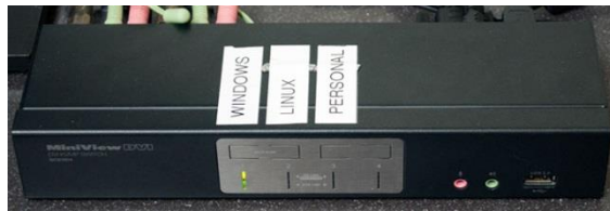
Figure 4. Four-channel KVM switch. This is the switch to select different stimulus computers. It will switch video, audio, microphone, and USB to one of the computers.
