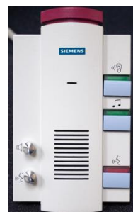
Figure 7. Siemens intercom. The button with a music symbol is used to turn on and off the audio signal from computer. The LED on it indicates on/off status.
