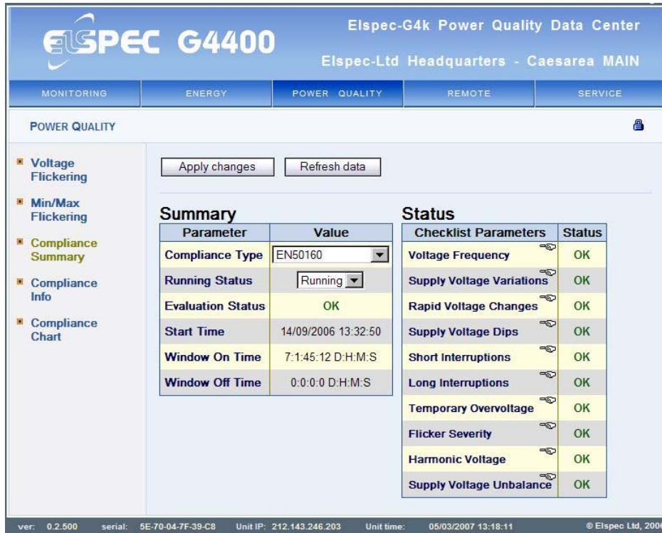
Figure 18: The Power Quality Compliance Summary
