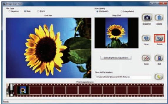
To manually adjust the image brightness and color level, click on “Color/Brightness Adjustment” icon. A pop up window containing Brightness bar and Color R, G, B bar will show up on screen and pulling the level bar to make adjustment.
