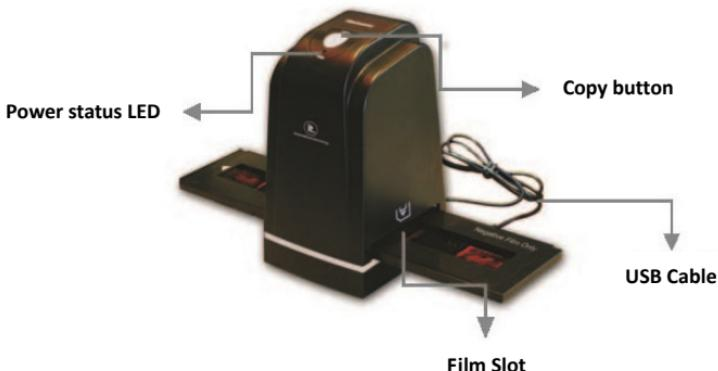
Plug in USB cable to computer without installing any necessary driver. When the status icon on the left button corner shows information "Your device is ready to use". The scanner is now ready to use. **Note:** Although the scanner is driverless, you still have to install the CD ROM so you can use the "Launch Image Scan Tool" application.
