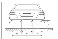
Fig.1 Mounting Height and Position of 4 Rear Sensors
