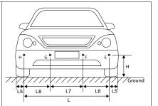
Fig. 2 Mounting Height and Position of 4 Front Sensors H = 50 - 80cm (20" - 32") L5 = 6 ~ 15cm (2" ~ 6") L6 = L7 = L8 or L6 = L8 = 0.3L, L7 = 0.4L
