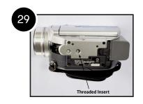
29. Check the bottom of your camera and locate the threaded insert.
