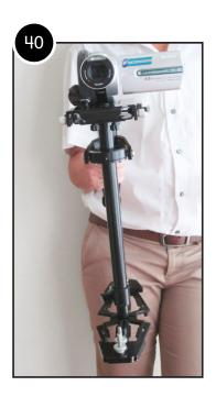
40. Once you're done adjusting the side-to-side balance, you might have to go back and tweak the front-to-back balance in order to get a true, fine balance of the of the entire system. You can either just do a visual check to judge for the correct horizontal balance of your GLIDE GEAR DNA-5050 or employ a lightweight bubble level (not included) to make sure.
