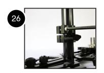
26. We have two ways adjust this alignment. The first and simplest method is to loosen the adjustment knob on the Telescoping Clamp and rotate the parts until they are aligned as seen in image #27; then, just tightening the adjustment knob back. Keep the I" of Telescoping Post visible below the Telescoping Clamp as before.
