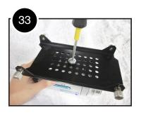
33. Place your camera on your lap or better yet, on a stable but cushioned surface—a folded towel on a table is a good example. Now that the Camera Plate is in position, use a screwdriver to affix the Camera Plate to your camera with the camera mounting screw and the 1/4" washer pair.
