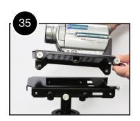
NOTE: If the Camera Plate can be easily rotated on the base of your camera even when you have adequately tightened the camera mounting screw, and you don't feel comfortable tightening the camera mounting screw some more, then you should consider using some kind of flexible "gasket" between your camera base and the Camera Plate. Some materials you can use are rubber tape or a flat piece of rubber you can easily find at home—you can, for example, cut up a piece of old rubber household glove.
