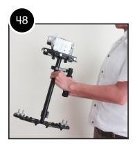
48. In the operation of the GLIDE GEAR DNA-5050, you will not be able to use the viewfinder. Putting your eye right next to the viewfinder's eyecup will hamper the stabilization capabilities of the GLIDE GEAR DNA-5050. It is best to use the camera's built-in LCD monitor as shown in image #53. Another option is to attach a separate external monitor directly to the Base Platform. This monitor "mounting hole" can be found at both the front and back edges of the Base Platform.
