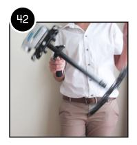
In short, if your GLIDE GEAR DNA-5050 is vertically balanced, your camera will remain level and the Central Post will stay vertical unless intentionally positioned otherwise. A vertically unbalanced GLIDE GEAR DNA-5050 will swing about and pendulum when you walk, run, or turn.
