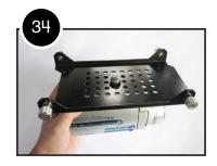
34. PROGRESS CHECK: Your camera and Camera Plate should now be securely attached to each other as shown in image #34.
