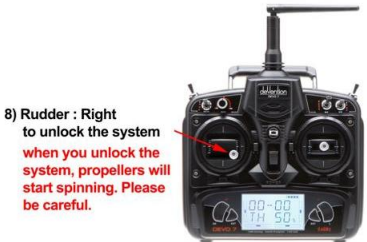
Mode 2 Transmitter (Left Throttle Stick)
