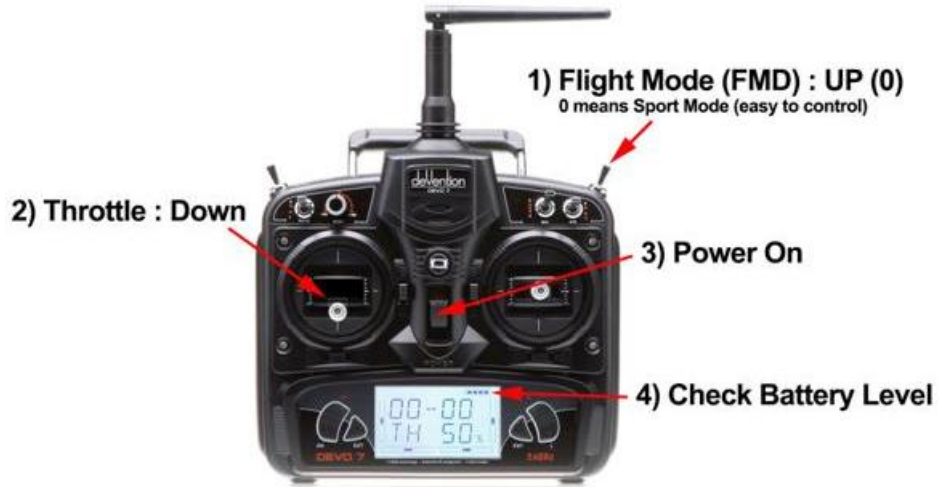
Mode 2 Transmitter (Left Throttle Stick)
